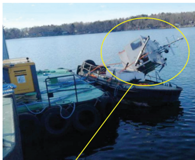
Tug wheelhouse torn from attachments
